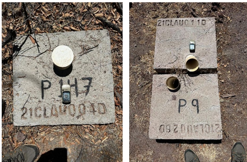
Figure 12-1 Collar Monuments for Holes 21CIAU004D, 21CIAU026D and 21CIAU011D
